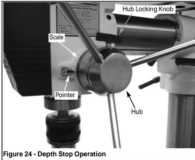
Figure 24 - Depth Stop Operation
