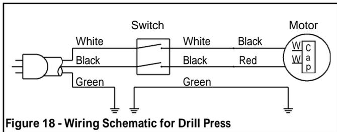
**Figure 18 - Wiring Schematic for Drill Press**
