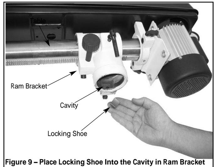
**Figure 9 – Place Locking Shoe Into the Cavity in Ram Bracket**
