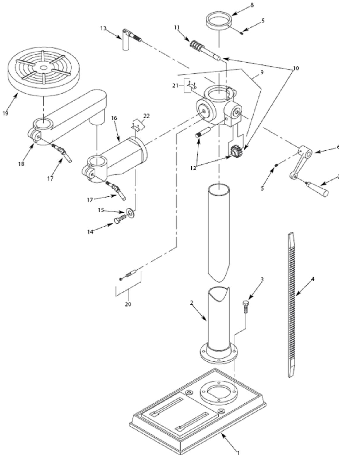
Figure 27 - Replacement Parts Illustration for Base (Model ZQJ3116A)
