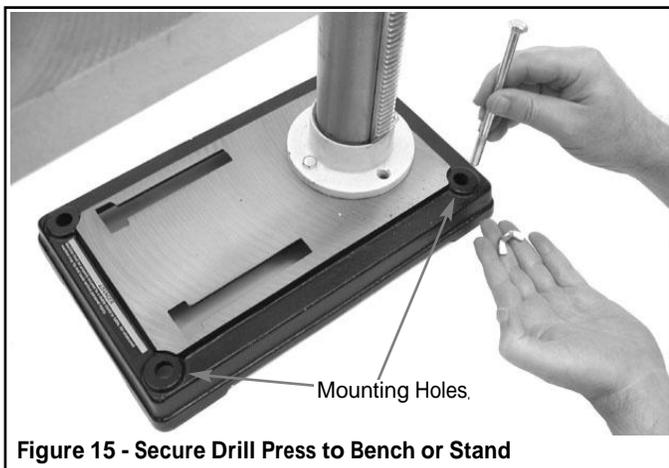
Figure 15 - Secure Drill Press to Bench or Stand
