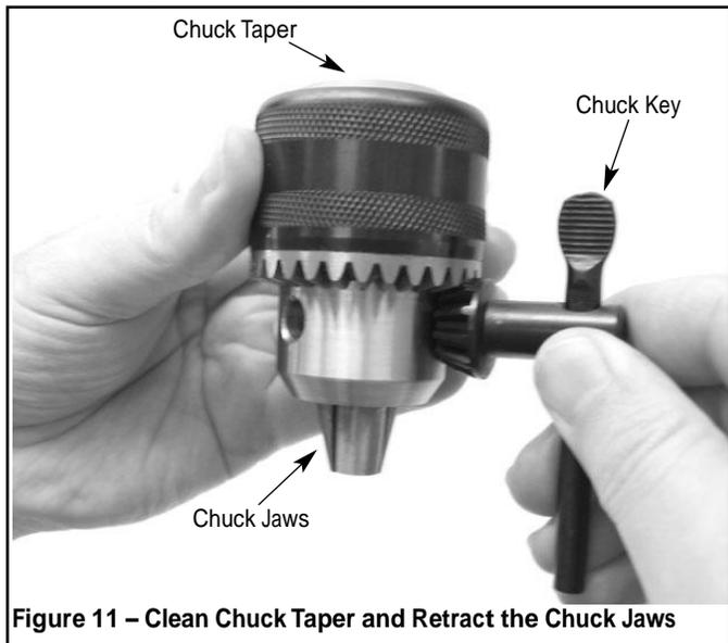
Figure 11 - Clean Chuck Taper and Retract the Chuck Jaws
