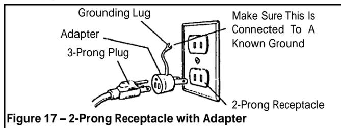
Figure 17 - 2-Prong Receptacle with Adapter
