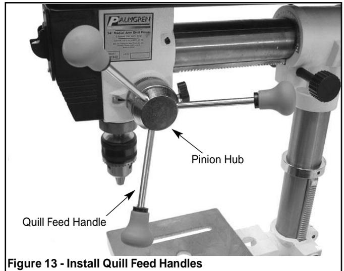
Figure 13 - Install Quill Feed Handles
