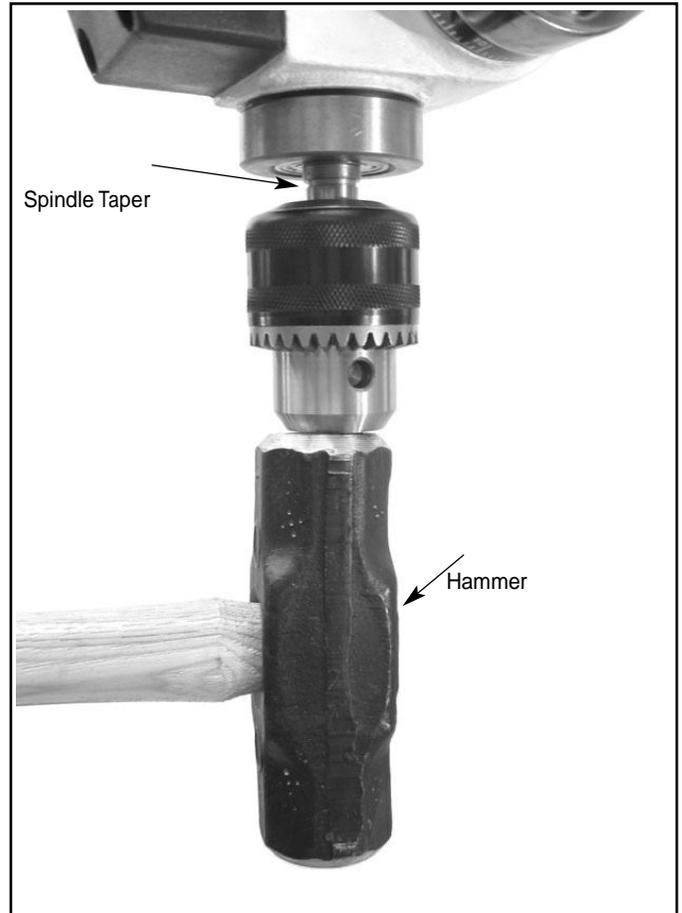
Figure 12 - Secure Chuck onto Spindle
