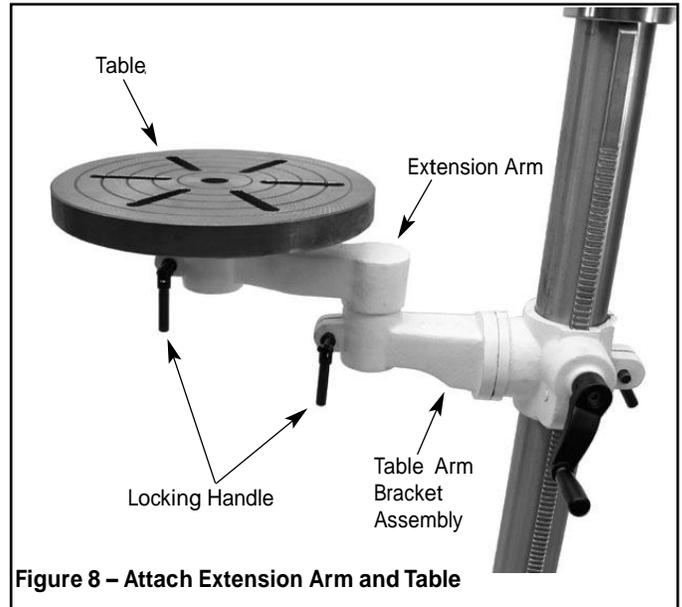
**Figure 8 – Attach Extension Arm and Table**
