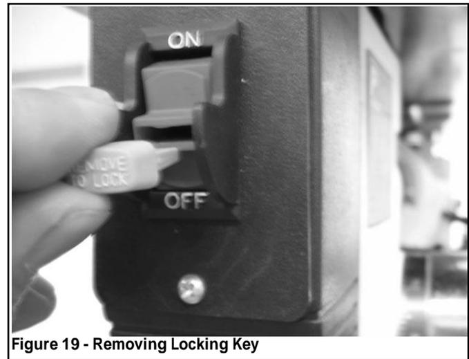
**Figure 19 - Removing Locking Key**
