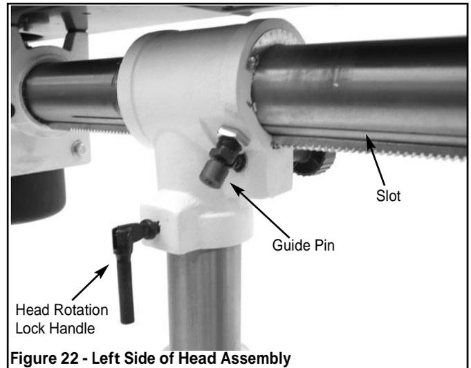
Figure 22 - Left Side of Head Assembly
